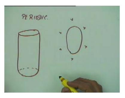
If we remember we had defined periodic curves and for a closed periodic curves, if we had an array of points like this, a closed curve or the smooth curve like this. Similarly we can define periodic surfaces and we can define closed periodic surfaces which can be totally closed surfaces. For example we can also have surfaces like this, this is closed in one direction open in the other direction, periodic in one direction and non-periodic in the other direction and so on.
