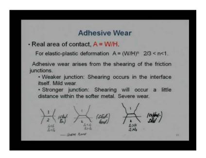
We will be studying this slightly lesser after sometime on when we come to the seven day slide of this of course,, of this lecture, but, let us quantify this wear mechanism or how the adhesive here of this. Whenever we want to quantify were like a wear volume or rate of wear, always is start with a real area of contact because of wear generally occurs at a area of contact. If there is no area of contact there will not be any wear..
