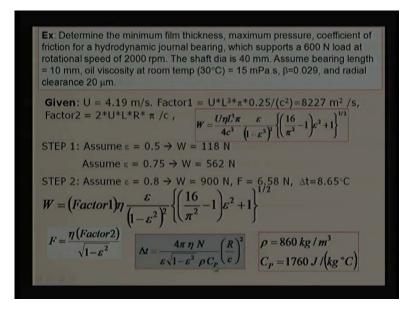
What this example means see in this case we are trying to find out number of bearing parameters, see its determined estimate or calculate minimum film thickness maximum pressure coefficient of friction we are not done coefficient of friction, but we know if we are able to estimate friction force and we know the normal load take that ratio F by W that is going to give me the coefficient of friction.
