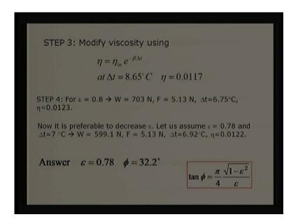
Now, once we know the temperature raise we can use this to find out what will be the viscosity, what will be the operating viscosity, that is viscosity is given as this is defined eta in is already known, beta is defined, delta t we calculated that is going to give viscosity as 11.7 mille Pascal second, in our calculation earlier we assume this is a 15 mille Pascal second, so almost 20 to 30 percent change in a viscosity.
