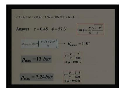
So, I can find out, I can close this example with extensity as a 0.46 or extensity of 0.45 both the options are open to me this is giving me high load carrying capacity, that is giving slightly lower load carrying capacity. So from conservative point of view I can choose this or for the continuity we say no we do not require too many iterations then iteration is itself is giving a reasonable good results (()) choose those results.
