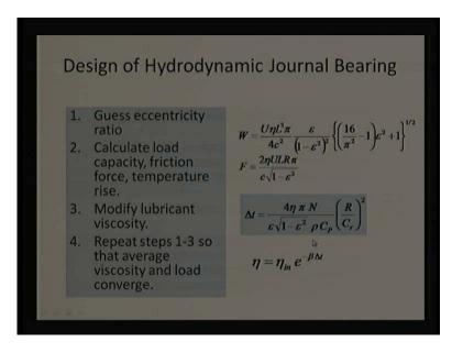
Now, we can think what we have done we have derived the relation for load relation for flow, relation for friction, relation for temperature and flow incorporate the relation of sorry temperature involves the relation of the flow that is why, we say how to do design first guess extensity ratio extensity ratio been guess may be 0.5 will be an initial approximation.
