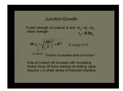
We can substitute those values sigma y is equal to sigma one minus sigma two and if I use a shear strength approximation we say that shear strength is generally fifty percent of yield strength. Depend on the which theory I am using or which component maximum shear stress or Tresca theory I am using. If the Tresca theory then this is will be the .577 sigma y while one might say that will be .75 .7577. While in case of Tresca theory it will be 50 percent of yield strength.
