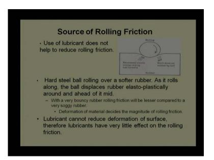
So, we will consider only the elastic case surface. Elastic itself is going to give coefficient of friction. So, to demonstrate that, there is diagram which shows that the roller rolling in clockwise direction. When it start rolling what it will be what happen to the material it will be going to the some pressure and if there is a rubber material then there will excess deformation of surface.
