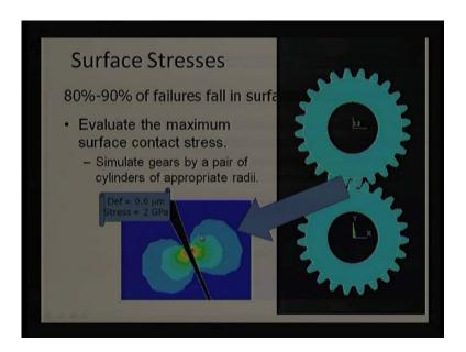
Now, when we were discussing about the bending value and surface value, how to say that tribology plays more important role compared to the mechanical engineering, as a bending value accounts to 10 to 20 percent of overall gear failure, why? Surface stresses, surface fatigue counts almost 80 to 90 percent of values of the gears.
