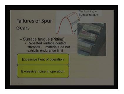
So, this is a thing, we are talking about the values and this is a typical picture of surface fatigue value of the gear. I can see there are number of bits for lesser or below the pitch circle radius, this portion, this portion, this has small pits (Refer Slide Time: 7:10). So, this gear is a spur gear, it is getting number of pits on flank or tooth flank, that is surface splitting failure of the gear tooth.
