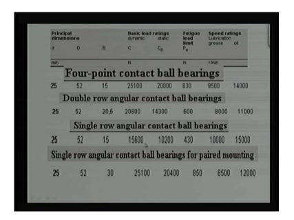
If I compare all these bearing what we say the 4 point contact ball bearing, double row angular contact bearing, single row angular contact bearing and single row angular contact bearing for the paired mounting for the tandem mounting whatever we show that pervious slide the paired mounting and tandem mounting. And for same diameter of the shaft we say assuming that these bearing is going to get mounted on 25 mm diameter, all the bearings are 0 5 C that is why I have shown here d 25, 25, 25, 25.
