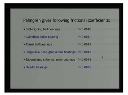
This slide shows a comparative study among the coefficient of frictions, you can say the coefficient of coefficient of friction f, for self aligning ball bearing is given as a 0.001, coefficient of friction for needle roller bearing is given as a 0.0045, for other bearings
