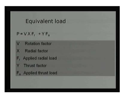
So, V is a rotation factor, with the inner ring is rotating or outer ring is rotating, if there is a rotation of outer ring, V factor will increase or we say that, impose low is going to be increase, if we are allowing outer ring to rotate and inner ring to be stationary. Coming to the X factor is a radial factor is a fraction, which need to be multiplied with a radial load F r is a radial load similarly, Y is a thrust factor need to be multiplied with a thrust load.
