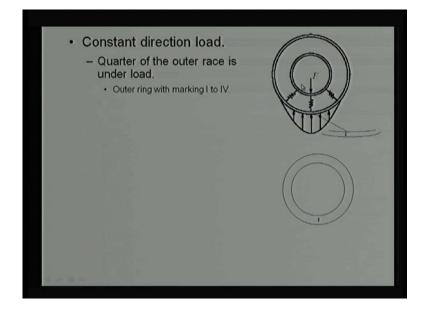
Then we found there was some clearance between the bearing, bearing was not preloaded and whenever there is clearance in a bearing. Only some portion of bearing will be loaded, it is not a complete bearing which is loaded. And something like that these are the inner ring, there is a outer ring and assuming there are rolling element in between that is spring connection shows the rolling element in between.
