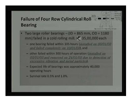
And to start I am discussing about case study in which we did for the one of the industry. What we call is the industry related to the rolling mill system. That figure shows, this is the rolling mill function is to reduce the thickness of sheet may be say thickness may be initially around 10 m m and we want reduce this thickness with 3 m m or 4 m m.
