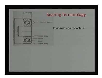
Four main components are inner ring, rolling elements, cage and outer ring. When we are requiring this kind of inner ring and outer ring and there is a separation by some rolling element. So, there is a possibility the inner ring is rotating or there is a possibility outer ring is rotating, any arrangement is possible.
