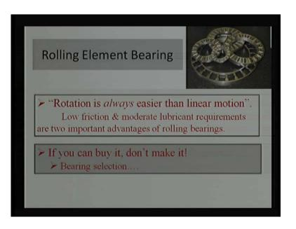
Another thing which is important for the rolling element bearing is a standardization. These bearings are mass produced. They have very good surface of its, and they work with elastro hydro dynamic lubrication mechanism. As these bearings are produced in mass, the cost is relatively cheaper assembling and disassembling is much easier. And that is why we say if we can buy something why to produce it.
