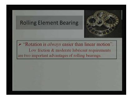
Reason being, they operate on the rolling motion and we always prefer rolling motion compared to linear motion. What we say rotation is always easier than linear motion, reason being low friction and moderate lubricant requirement.
