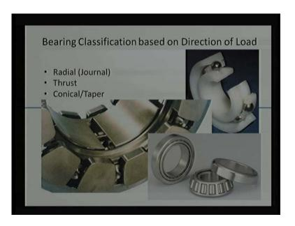
We can think about as a arrangement is shown here, we can think about classification of bearing based on the direction available, this is color radial bearing apply load is generally in radial direction perpendicular to the axis, if I assume that is a axis passing at the center of this inner ring, now the load which is perpendicular to that, that is going to develop a radial stress.
