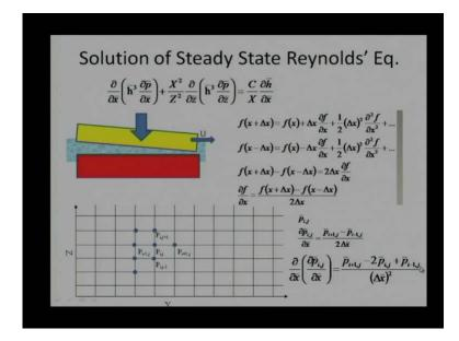
We consider only the steady state Reynolds equation, where the time dependent term was neglected. The dh by dt is negligible for a steady state Reynold's equation; and we considered rejection as in viewing the surface is rigid there will not be any pressure generation due to variation in surface velocity. Surfaces are rigid, u is constant it is not a function of any space variable.
