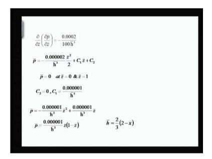
While in the present case integration is much faster you can simply take out h cube rearrange this equation in this term and this is a constant integrate 2 times after 2 times integration what we get here z bar square divided by 2 plus integration constant at the integration constant first we can multiply with the z bar and then integration constant 2. So, we have a 2 integration constants and we know we have a 2 pressure condition p 0 at z is equal to 0 p 0 at a z is equal to one.
