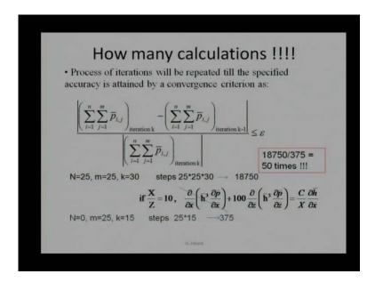
And for we can use a boundary condition as an initial condition not boundary condition initial condition P i j is 0 at all nodes, then this is a convergence criteria we are have been we are using. We say that at any iteration k whatever the summation pressures or non dimensional pressures for all the nodes, you say that when node vary from; in x direction 1 to n.
