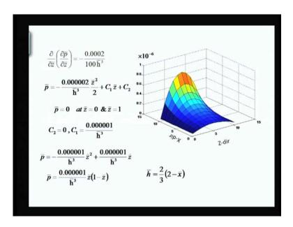
Only thing is that dimensional was a dimensions was to vary different in first example or previous example, we considered x dimension may be much lesser compared to the z dimension while in present example we are considering x dimension are much larger compared to z direction.
