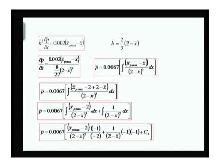
To do that and we require expression of h that is already we determined that is a 2 by 3, 2 minus x bar substitute this rearrange equation we know is h bar cube. So, cube of 2 two will turn out to be a 8, cube of 3 will turn out to be 27 and this will be 2 minus x bar cube. We can rearrange this equation something like this and then integrate it you say, x bar x bar max minus x bar integrate with the respective x and this is also depending term, this is a function of x bar.
