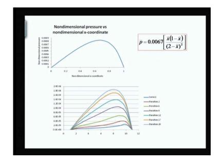
When we do that, we get a pressure profile something like this. This is a simple, you just substitute value get a pressure value, no iteration, in one iteration we are getting the solutions. So, this is maximum value is coming where here 0.7; that means, the node number 8, node number 11, node number 10, node number 9, node number 8 and this is a what we same value same similar expression or we say that same location we got a
