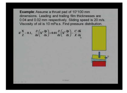
We can, I will this example, I will cover in next lecture, but, for the time being I can show what we expressed in previous slide 1 example related to that. I am assuming there is a first load or load perpendicular to the axis is coming over it. There is 1 plate with stationery plate, 1 sliding plate which has a velocity u and this velocity in the present example is given 20 meters per second, which is very, very high velocity.
