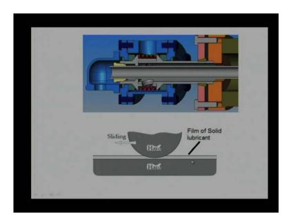
We can use carrier fluid very when we are relying on this kind of coating, can use carrier fluid on that along with the solid lubricant. Now, one of the major groups of the solid lubricant is a polymer. We say that the polymers are suitable to bear the light loads if you applied a load with high magnitude load, then they have a coefficient of friction.
