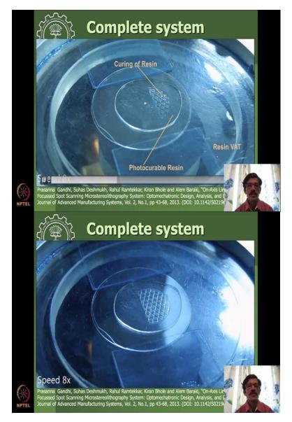
So, once the component first layer gets printed like this. So, this is a layer getting printed. So, there is a continuous motion in the Y direction and stepping motion in the X direction that is happening here and this component gets slowly slowly developed here. So, this is like a hexagonal kind of a comb kind of a structure honeycomb kind of structure.
