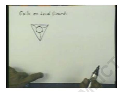
if you take the three feet on the ground the convex hull of that that is the minimal convex head which includes those three points is the triangle fine
