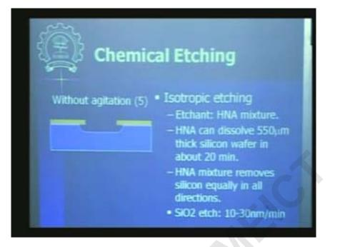
And now isotropic etchant it will produce a surface of the slot okay so you can observe here that there is some kind of a undercutting happening here okay
