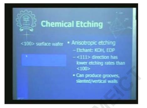
So all the crystals are aligned in such a way that their one zero zero axis is perpendicular to the surface okay
