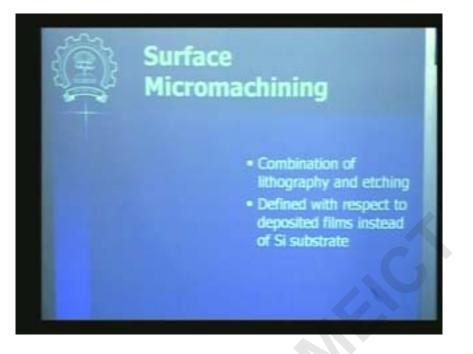
Now let us see surface micromachining which is the next process so it is the combination of lithography and etching processes okay
