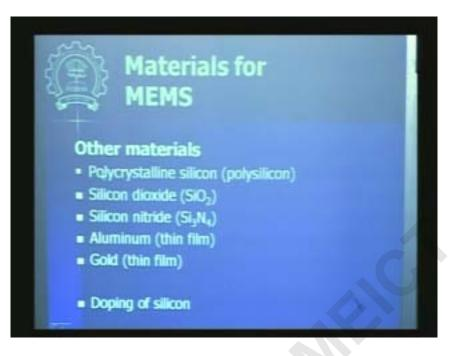
We can have look at polycrystalline silicon or it is called polysilicon it is a gra granular form of a silicon okay it is it is not crystalline it is has grain and grain modrincs and like that and then silicon dioxide silicon nitride aluminum you can have gold you can have okay
