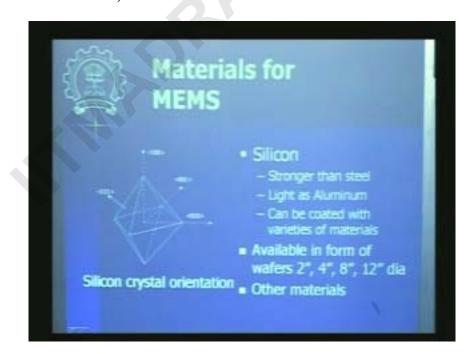
So firstly what are the materials that are used for this MEMS okay the primary material is silicon because this technology is driven by VLSI technology which is silicon based chip fabrication technology okay
