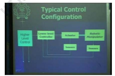
so this is the typical control configuration for the robot manipulator ok i mean these part you can say it is a general control configuration for any dynamical system but typically each axis of the robot will have its part ok so you have this load level controller which is actually controlling the actuators the sensors can be giving the feedback from either actuator or actual robot manipulator ok
