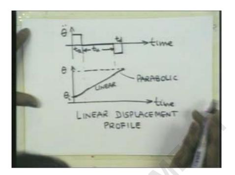
All the relations that I will use in this strategy are based on the high-school physics relationship that you must have worked out. Final velocity is initial velocity plus acceleration time, and the distance traveled is initial distance plus velocity plus half at squared.
