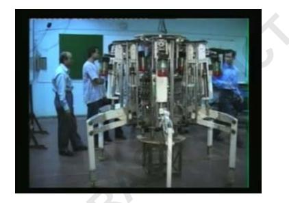
the size of the robot in comparison to humans around it. You can have a look; you can see the motors, the red and green ones are the motors; then there are ball screws which are used. Now you can watch the walk; you can very clearly see the robot lifting up three legs, throwing them forward in order to move—the front two and the rear one leg are moving. It is a very slow motion because the robot is very heavy; this was the first walk it took.
