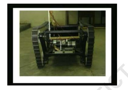
You can see a couple of motors driving through chains, the tracks. Here is another view (Refer Slide Time 18:18 min); you can see the battery—all robots are more or less required to carry their
