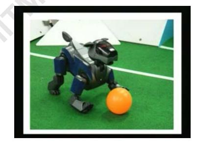
and then it has got the sound sensors, which can receive sounds and can determine from which direction the sound is coming. It has many other sensors built in to the system in order to enable it to behave almost like a real puppy. This picture shows the Ibo playing football; the ball is colored orange in order to identify the ball to the Ibo dog. It is a very popular one and it is now being used as an entertainment pet by senior citizens.
