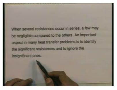
A statement is as follows; it says - when several resistances occur in series as in a long composite cylinder with two solid materials; we had four thermal resistances - one associated with the  $H_i$ , one associated with the thermal conductivity  $K_1$ , one associated with the thermal conductivity  $K_2$  and finally the one associated with the outside in terms
