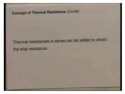
Thermal resistances in series can be added to obtain the total resistance; when we have many resistances in series, the thermal resistance - total thermal resistance - is the sum of the individual thermal resistances. Now with this backdrop, let us look at a composite situation. A composite situation is one in which we have a number of thermal resistances in series.
