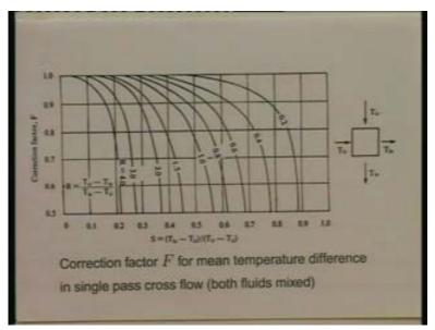
And then finally, here is the correction factor F - results for correction factor F plotted for mean temperature difference in single pass cross flow for the case of both fluids mixed; similar results but of course numerical values are different. So, depending upon which cross flow case you have, you will go to the appropriate figure and read off the values of S that is the point I want to mean.
