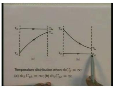
This is the figure a corresponding to m dot h  $C_{ph}$  tending to infinity; the temperature on the hot side doesn't change or this could be a vapor condensing. The temperature on the cold side is increasing. The b is the case of m dot c  $C_{pc}$  tending to infinity so the
