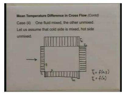
One fluid mixed, the other fluid unmixed. Let us assume the cold side fluid is mixed and the hot side fluid is unmixed. Now what we are going to get is something like this. This is our cold side fluid. Let me draw its temperature profile. This is our cold side fluid uniform while entering which is  $T_{ci}$  and this is where the fluid is entering, cold fluid
