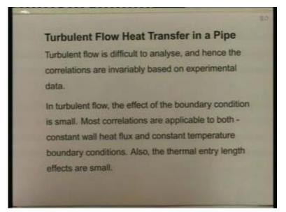
Unlike laminar flow because of the eddies form during turbulence and turbulent mixing, turbulent flow is invariably difficult to analyze; much more difficult than laminar flow and hence we obtain information for turbulent flow essentially from experiments and all the correlations or almost all correlations which we have for turbulent flow are based on experimental data. In a way turbulent flow is slightly simpler because in turbulent flow the effect of the boundary conditions are small.
