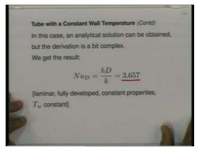
Again notice that this is for a circular tube in which the flow is laminar. Fully developed fluid can be assumed to have constant properties and the wall temperature is constant. By fully developed we mean both fully developed velocity profile as well as fully developed temperature profile.
