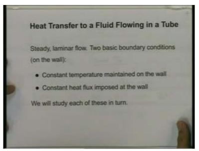
Near the end for the previous lecture, we were about to study heat transfer to a fluid flowing in a tube and we said we would look at the constant temperature boundary condition and the constant heat flux boundary condition on the wall.
