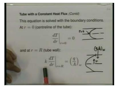
One is at the center length; we have seen that whenever the flow is fully developed or even otherwise the temperature profile is symmetric with respect to r equal to 0 and we use that fact to create a boundary condition at r equal to 0. That is the centerline of the tube which is dT by dr at r equal to 0 if 0. So the temperature profile at the center is locally flat that is what it means.
