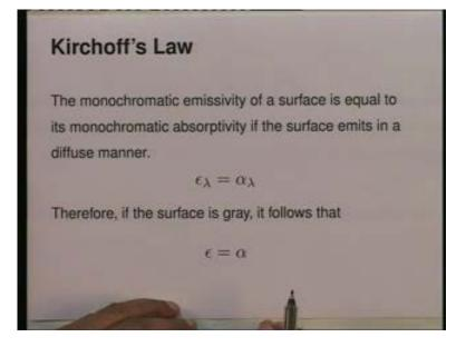
Kirchoff's law states that the monochromatic emissivity of a surface is equal to its monochromatic absorptivity if the surface emits in a diffused manner. Kirchoff's law is a very powerful statement relating the emission characteristics of a surface with the absorption characteristics of surface. Kirchoff's law I repeat is a very important law -
