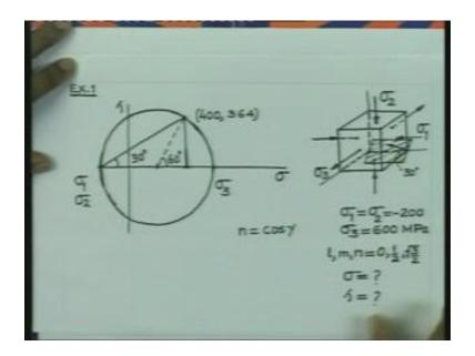
Let us consider that, this is the principle, stress direction 1, this is 2 and 3. The magnitude of the two principle stresses, sigma 1 and sigma 2 are minus 200 MPa and sigma 3 is 600 MPa. So, in this case, what is needed is that, find out the stress on a plane, which is making an angle as whose outer normal is making an angle of 30 degree with the sigma 3 directions. And 60 degree with the sigma 2 directions.
