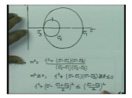
So, therefore we can now draw the circle, which is going to be showing the spread up all the tau and sigma. So, this will indicates that, all the points, all the combination for stresses. And stresses, I am going to lie on this circle, the center is here and radius is this. It is on this circle or within the circle.
