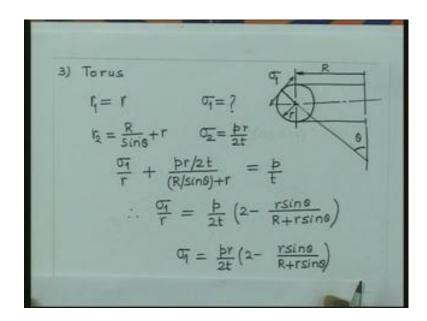
Let us consider the case of the torous. This is something very typical. So, in the case of a torous, we have the hoops stress which is going to act perpendicular to the plane of the paper. That space is going to be given by sigma 2, which is p r by 2 t very easy to determine. Now, we are interested in finding out the axial stress sigma 1 acting like this. And this axial stress, obviously the radius of curvature for that is this r.
