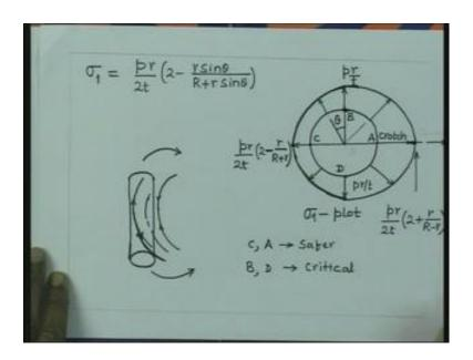
Let us write once again, p r by 2 t 2 minus r sin theta by R plus r sin theta. So, we draw the circumference of the cross section. Let us write this point to be A. The vertical point vertically top most point is B and this, for this point from this center. So, center of curvature is somewhere this side. And this bottom most point is let us say D. And our reference direction is this one. So, this is what is? theta direction.
