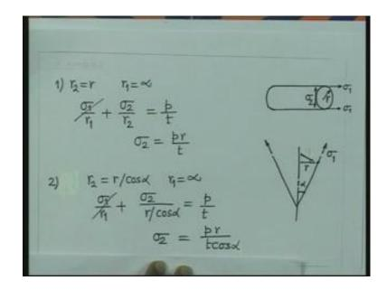
And this cylindrical shell is of radius r and the wall thickness t. We have the stress sigma 1, acting in the axial direction and circumference stress is sigma 2. And therefore, this r 1 in this case, which is infinitive and r 2 is going to be r. So, if I now apply the formula, sigma 1 by r 1 sigma 2 by r 2 is equal top p by t. And since, r 1 is infinitive this term goes off. So, you have now sigma 2 by r is equal to p by t.
