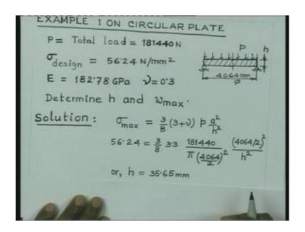
Let us now consider one example, on the design of a plate, it is a thick plate of uniform height h for thickness h, its diameter is 406 per millimeter, the total load which is uniformly distributed, which is given by 181440 Newton. As in specified that the design stress of the plate is 56.24 Newton per millimeter square and E for the material 182.78 GPa, it is steel. And poisons ratio is point 3, what is needed is that calculate the thickness h and the maximum deflection of the plate.
