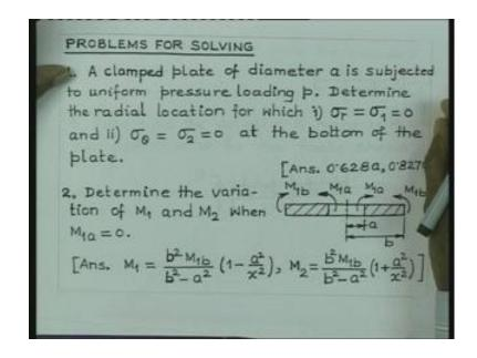
A clamped plate of diameter a is subjected to uniform pressure loading P. Determine the radial location for which, sigma r which is nothing but sigma 1 equal to 0. And sigma theta equal to sigma 2, 0 at the bottom of the plate. So, therefore, determine the location where, sigma 1 is going to be 0 and sigma 2 is going to be 0. Obviously a plate which is subjected to loading at the top, you know that for a clamped plate the stress varies from 0 from positive to negative.
