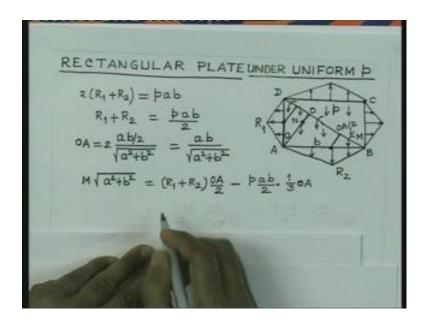
Let us consider that the height is a and this width is b. And it is subjected to uniformly distributed load. The plate is simply supported at its outer boundary and the pressure loading is P; obviously, the reaction over the boundary it is not going to be uniform as in the case of circular plate. Here, the center of loading is exactly at the center of the plate and this one, the middle points of the size their closest to the center of gravity and therefore, what you find is that.
