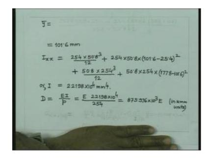
If we do that will give us y bar as 101.6 millimeter. So, therefore, the CG is located at a distance of 101.6 millimeter of the top. Now, if I know that I can now calculate the moment of inertia of this section about Ixx, so if you calculate Ixx. We can now consider this segment, which is of dimension 254 height 50.8. So, therefore, we will have the moment about its own CG parallel to x axis is 254 into 50.8 cube by 12.
