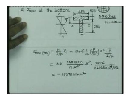
So, therefore, if we can write now this maximum stress for this problem is going to be at the top is nothing but M this I per unit length. So, therefore, I by P into Y 1 because this moment is given per unit length, so therefore, this has got to be also per unit length. Sigma maximum is equal to M by I by P into Y 1. So, if you are calculating the stress at the top fiber you must think of distance Y 1 of the top fiber from the centralized location.
