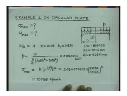
So, the problem is shown here, this is the plate the cut out at this center is of radius a and outer radius is b, the load is uniformly distributed, total load out of this uniform distribution is 181440 Newton. And as I said that this inner radius is one fourth of the outer radius. Now, let us see what happens to the maximum stress and the deflection. So, these are the two things to be calculated.
