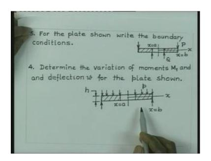
Similarly, you can consider a plate which is loaded like this, the radii of the plate is x equal to a to x equal to b. The loading at the outer edge is P per unit length and loading at the inner edge is Q per unit length. For this plate write the boundary conditions. For a plate like this, where it is supported at the edges and distributed loaded who are the annular area, which is from x is equal to a to x is equal to b. Determine the variation of
