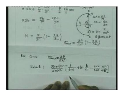
So, if we now to a equal to 0 will have sigma max is equal to 3 p by pi h square. So, that is the maximum stress, which is going to occur at the bottom fiber, it is going to be tensile stress and if it is of the top fiber it will be going to compressive stress. You might be interested in trying to know, what is the exact value of this stress if, we go rigorously for the analysis.
