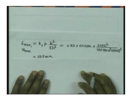
Delta maximum or it will be W maximum is equal to k 1 into p b 4 by E h cube. So, W maximum is k 1 p b 4 by Eh cube. So, if I substitute the value that is the value of b and this is the value of E 182.78 into 10 to the power 3 and this is 35.65 cube. And on simplification we get this thing as 25.5 millimeter, the deflection in the earlier case we had only 20 millimeter. Now, the deflection is increase to 25.5 millimeter.
