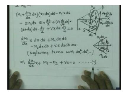
So, this is a portion of the plate that we would like to focus our attention and we will consider now our radial directions to be x and then this element is symmetrically placed above the X axis and let us say that it is making an angle of d theta at the centre So, this is our Z axis. Now, bending moment is not going to remain constant in general and therefore, let us consider that on this face theta face, which is perpendicular to radial face this is radial direction.
