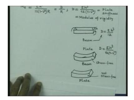
And this quantity we try to write like this: Mx is equal to Eh cube 12 into 1 minus nu square into R and we write this thing as D by R, where D is equivalent to E into I and D is equal to E h cube 12 into 1 minus nu square. And this is known as plate stiffness Modulus of rigidity. So, let's just have something to consider here. If I had a beam like this.
