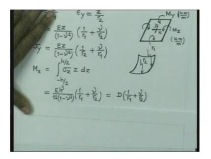
So, generally its unit will be Newton meter per meter. Similarly, M y we apply in this direction, which is again having unit Newton meter per Meter. So, we can now write if the curvature due to M1 let us, say that we have curvature equal to r1 and the curvature that we get in this direction is equal to let us say r2. Then, we can write the strain in the X direction is equal to z by r1 and similarly, epsilon Y is nothing but z by r2.
