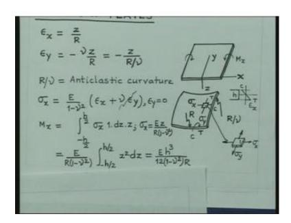
Let us consider a rectangular plate which is very thin. The height is small compared to length or the width. When, you try to apply bending load to such a plate. Let's, say we apply the bending load in the X Z plane like this and we would like to indicate this moment by M x. So, when you do that what you find is that we are trying to have bending generated like this. The surface should have curvature like that and you find that.
