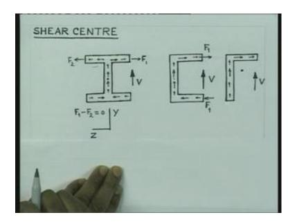
You can have a cross section of I type, C type, L type. When, you try to consider bending of such beams of such cross section. Suppose, a shear force is acting on the section like this, then you are quite clear. That the shear stresses that acts, due to v are going to be like this. We will have maximum shear stress near the centre of the wave. And then it will gradually reduce in magnitude, as we go away from the centre portion.
