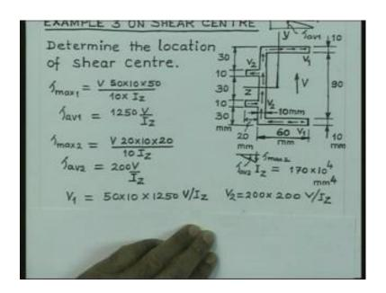
So, it is a section which is like C, but then we have some flanges also on the other side. It is not exactly C type section and wall thickness everywhere is 10 millimeter and this height is 100 and 10 and this is 60 and this flange length is equal to 20 millimeter. The cg of the cross section is somewhere here and this z axis is an axis of symmetry, y is really the axis which is not a symmetric axis.
