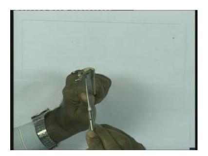
If I put a load there on the cross section, you see it is twisting, it is twisting. I put a load there at this point it gets rotated.
