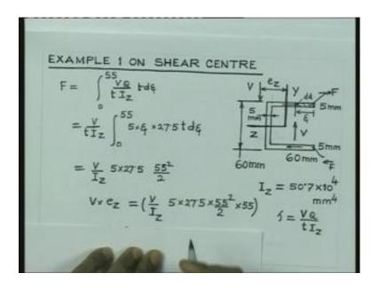
So, let us consider example 1 on shear centre. We have a cross section given here. The flanges are of dimension 60 millimeter. Wave is also of dimension 60 millimeter and the wall thickness is 5 millimeter everywhere, and so therefore this is 5 millimeter and so also this is also 5 millimeter. Now, I z for this cross section has already been calculated
