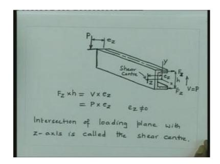
So, we have a beam with C section here. So, this is the beam we have. Now, we are, what we have shown you is that the axis of the cross section are as follows. This is your y. This is z axis. Now, if you put a load parallel to this y x plane. So, parallel to y x plane. Let us say that we put a load here, somewhere there, you just think of it that we have put some member, welded some member and we are putting a load there. Then in that case, this is going to be at a distance.
