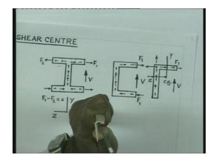
So, therefore, this corner is the shear centre of this cross section. So, now we will solve some problems to have further understanding of this one.
