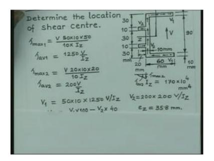
So, now I can write the balance equation v total shear force multiplied by e z is equal to v 1. And this distance from this to this middle is nothing but 100, so that is the moment. And v 2 is the other force and here the distance is it is again from here to here is 40. So, therefore, that is the equation to calculate the distance e z of the loading plane and if you substitute this values of v 1 and v 2 here. On simplification you get e z equal to 35 point 8 millimeter.
