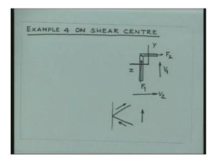
Even if you have a section like this, if you have a section like this, here again if you have a vertical force acting like this. The shear force stress is going to act this way and then their intersection point is here and you will find that, the shear centre is going to be passing through this point. So, this I think is you can easily establish. So, this is the section, now we are trying to keep it at an angle.
