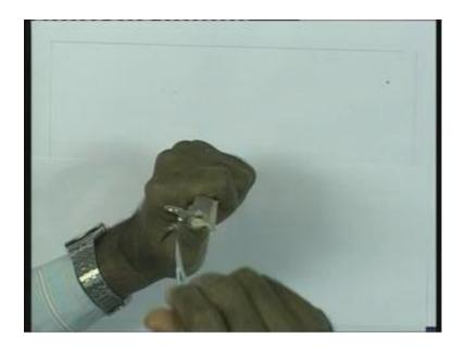
I have a section here, this is again made up of plastic. You see here, this is the section, which is like a c section. I have put some paper inside that is all. So, it does not have any stiffness.
