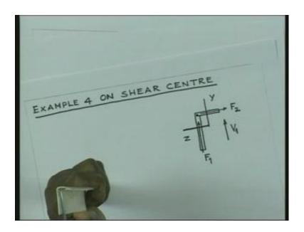
But, if I make to pass it through this point it does not get twisted. So, therefore, we must actually see that this load passes through the point of intersection here. Similarly, if you are now trying to consider. Lets the loading plane is like this, which is parallel to the other arm. So, then in that case again I am going to get forces like this F 2 and F 1. Of
