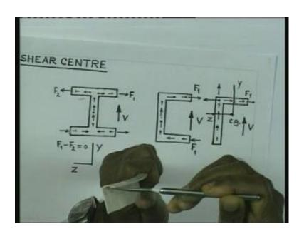
But, then if I apply the load at the junction, it does not get twisted.
