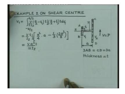
Let us consider another example. So, this cross section is shown here. It is like t and the orientation is like this, that you have one flange oriented vertically and this is another flange, but then this is the wave, which is a line with the z axis. And this AB and CD they are related this is 3 times AB. So, therefore, 3 AB CD is equal to A and this is equal to 3 A and this is equal to A and the distance of the two legs AB and CD is equal to a
