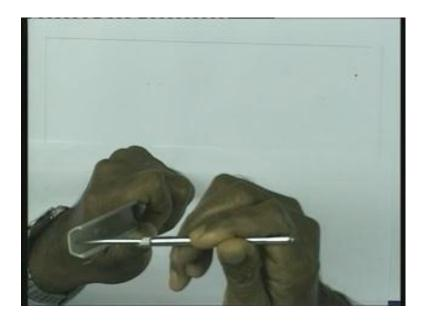
So, let us see, that if I now try put a bending load like this, this is the point. So, I am applying the load, you see that if I apply the bending load like this, on the cross section. There is no rotation of the cross section.
