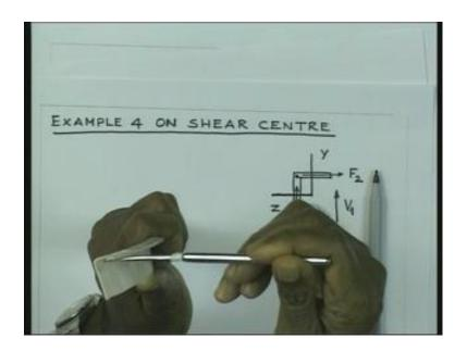
But, then if I apply the force which is close to the intersection point it does not get twisted it gets twisted. But, if I apply the force, so that one it does not get twisted, so therefore, for such L sections, always you will find that the intersection point is the shear centre.
