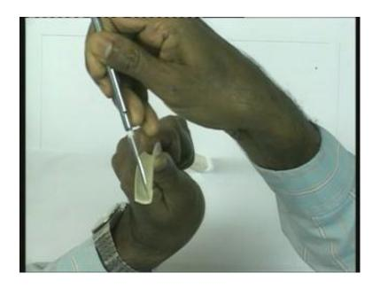
But, then if I put the load there, it does not get rotated. So, that is the point, which will be related to shear centre. So, let us try to do some calculations on this determination or locating this shear centre. How do you go about it. Let us get back to our C section.
