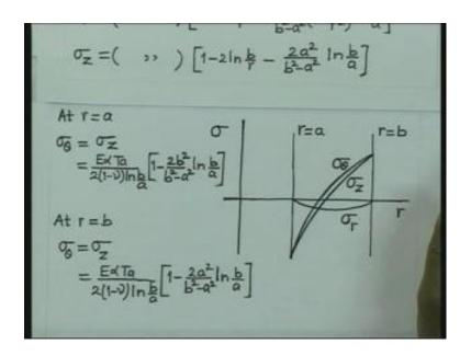
So, at outer radius it is going to be given by sigma theta is equal to again sigma z. And it is E alpha T a by 2 into 1 minus nu 1 n b by a, into 1 minus 2 a square by b square minus a square 1 n b by a, so this is the stress at the outer radius. So, this variations of the stresses, once you plot it looks like this. We have stresses plotted in this direction, radius in this direction. You will have this as the variation of sigma theta. This is the variation of sigma z.
