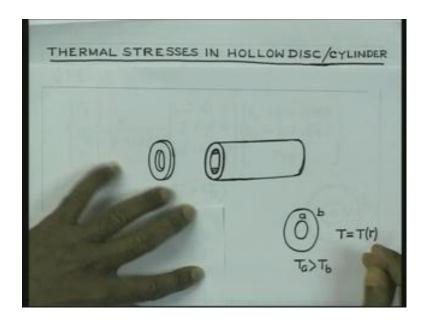
We would like to consider therefore, problem to be thermal stresses in hollow disc or cylinder. You could have a situation of this type or a situation like this. That is a pressure vessel or a cylindrical vessel, which is going to have temperature variation in the radial direction like this. And we would like to calculate the stresses. If we calculate the stresses for a situation like this, where there is internal radius and external radius.
