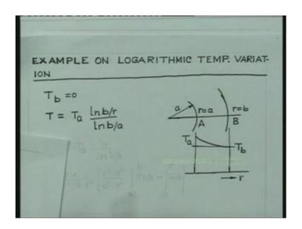
Let us consider that, we have the well known case of thermal. When heat exchangers are conducting or exchanging heat, you find that the wall temperature is going to vary from the inner wall to the outer wall. And this if we plot in this direction temperature. And in this direction the radius, then it is going to be like this. So, we have the vessel of radius r equal to a to r equal to b. And most often the temperature variation is going to be, if we take this as the data.
