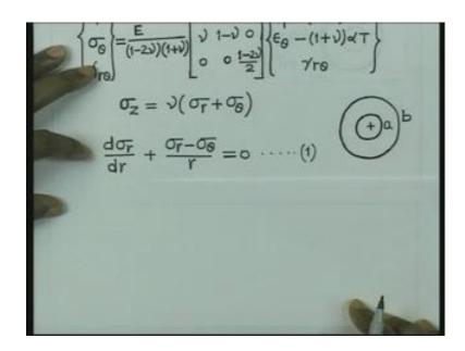
We derived the relationship, the equilibrium equation. The equilibrium equation for this problem also will be similar. And therefore, the governing equation for this stress distribution is given by d sigma r d r plus sigma r minus sigma theta divided by r equal to 0. So, that is the governing equation of distribution of radial stress and tangential stress. Let us consider this equation to be number 1.
