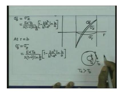
Let us, try to see whether it is tallying with our expectations, as we started saying at the beginning. If temperature here is T a, temperature here is T b. If T a is greater than T b, then we expect the inner fibers to expand more than the outer fibers. So, their expansion will be arrested or rather constrain by these lower expansion of the outer fibers. And hence, these fibers will be subjected to compressive stresses and since these people are trying to these fibers are trying to extend.
