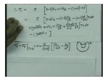
So, if you consider now, this typical cylinder here, just a cross section of it. You have the radial stress. There is no external loading acting on the inner wall. And therefore, the radial stress on this boundary is going to be 0. Similarly, there is no external loading on the outer boundary. So, therefore, the radial stress on the outer boundary too is 0. So, therefore, we can now consider that both the surfaces are free of any radial stress. Therefore sigma r equal to 0.
