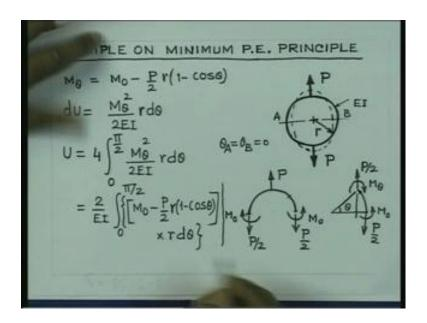
Now, we will consider 1 example on the minimum potential energy principle. These energy principles are very useful in solving equations statically indeterminate problems. So, let us consider application of the minimum potential energy principle for solving 1 statically indeterminate problem. Consider the case of a ring of uniform cross section let us say that the modulus of rigidity of the cross section is EI.
