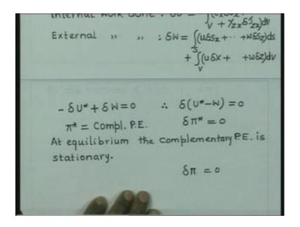
So, therefore, by the method of virtual work we would have delta u star and here in this is delta u star plus delta w equal to 0. And therefore, now we have seen that they are of opposite sign. So, we can write now delta. In fact, we find that this is negative work done
