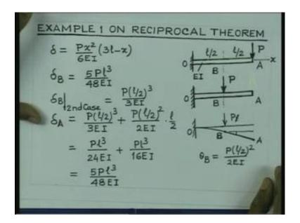
Now, we would like to consider some example, very simple example to illustrate the first example we will take it up like this. You take the example of a beam this beam is of length l it is subjected to a force P. And let us consider that the modulus of elasticity is E and the moment of inertia is I. So, therefore, the modulus of rigidity of the cross section is E into I.
