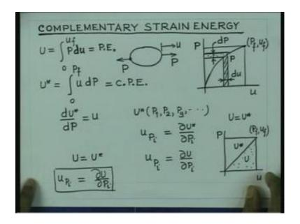
And this principle is a is obtained from the consideration of method of virtual displacements. Now, we would like to consider some other theorems. Before, we can do that we must introduce, what is known as complementary strain energy. You consider a component which is loaded like this. Now, if we consider that, this point is having a displacement equal to U when the other point is fixed. We can plot the load versus deflection diagram.
