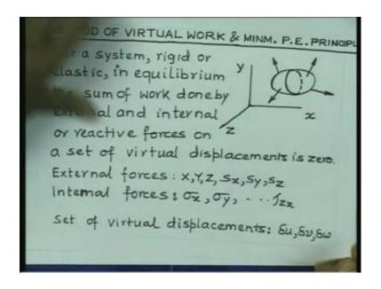
Now, according to method of, according to the minimum potential energy principle; for a system, rigid or elastic, in equilibrium, let us consider the method of virtual work, we would like to define it. For a system, rigid or elastic, in equilibrium, the sum of work done by the external and internal or reactive forces on a set of virtual displacement is 0. So, the method of virtual work is stated like this: for a system, rigid or elastic, in
