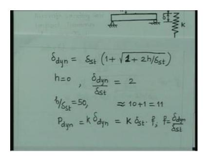
So, the dynamic deflection if you represent that this delta that come up because, of the drop is equal to delta dynamic is equal to delta static multiplied by 1 plus square root square root 1 plus 2h by delta static. So, we find that the dynamic deflection is always going to be more than the static deflection. And you find that when h equal to 0 delta dynamic, by delta static is equal to 2 when h by delta static is equal to let's say 50.
