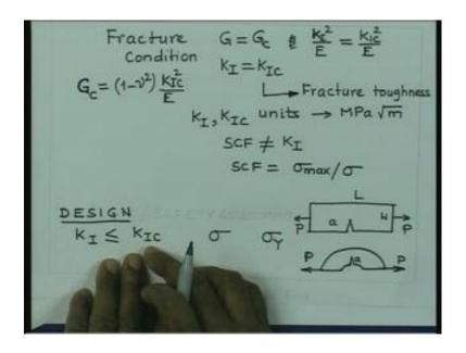
So, at the point of onset of fracture strain energy release rate reaches a critical value. Now, if G is given by Ki square by E if at the point of onset of fracture G reaches a critical value it is obvious, to expect that this KI also reaches a critical value. So therefore, at the onset of fracture KI square by E is equal to KIC square by E. So therefore, this is G and that is Gc. So therefore, at the point of onset of fracture we have KI equal to KIC.
