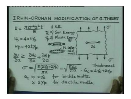
So, a modification to Griffith theory was proposed. So, that the theory can cater for some amount of plastic deformation taking place during the crack propagation this is known as Irwin Orowan Modification of Griffith theory So, this is Irwin Orowan Modification of Griffith theory, so we would like to talk about this Irwin Orowan modification now. If you consider a plate loaded like this and assume that there is a crack of size 2a.
