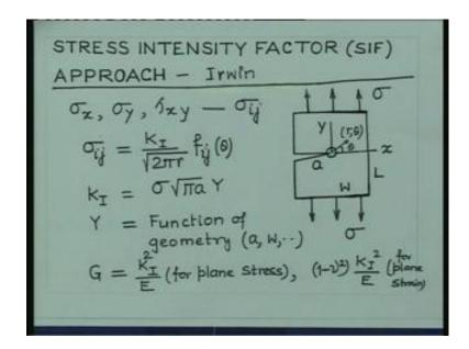
What Irwin did is that he consider the crack in the material and he analyze the stress and strains around the crack tip under the action of the loading and in a 2 dimensional problem like this. If the situation conforms to plain stress, then the stresses that are going to come up are nothing but 3 components: which are sigma x, sigma y and tow xy. So, let us represent them that these are nothing but the sigma ij stress.
