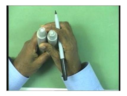
The other example that we were considering the other day is the failure of the aluminum specimen in the tensile test. And in this case, we saw that the failure was at an angle of 45 degree. We had the cup and cone failure. This is the cone and this is cup and this angle is about 45 degree with the loading direction.
