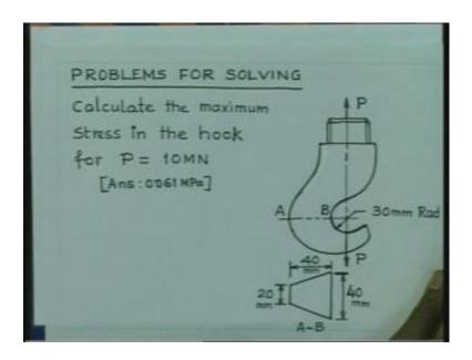
You have a crane hook, the dimensions of the crane hook. There is a radius here, which is just 30 millimeter. And this cross sectional area at A B is trapezoidal. Generally in this construction you will find that, the larger width is going to be at the inner radius. So, therefore, you have 40 here and 20 at the side.
