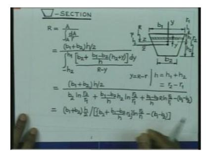
So, we will now look into how to calculate the eccentricity of a trapezoidal section. Consider the typical section to be as shown here. The center of gravity of the cross section is located here. As usual we consider that the radius of curvature of the centroidal axis is r bar. And the radius of curvature of the neutral axis is R. And we will show the extreme fiber ((Refer Time: 09:19)) i to be r 1 and r 2. The neutral axis is passing through this point.
