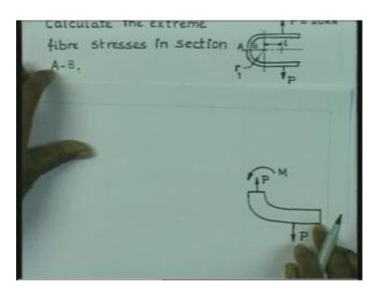
You can consider this problem, if I take this section A B. So, if I just consider a section like this, here in you have the force P is acting externally. And therefore, you are going to have a reaction force here P, which is passing through the centroid of the cross section. Then, you are also going to get a bending moment M.
