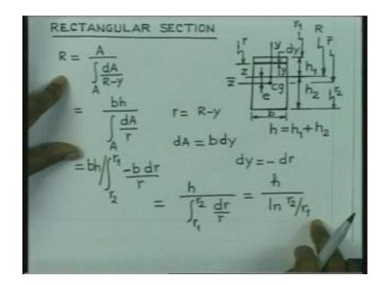
Let us consider the rectangular section. For the rectangular section, we have the radius of curvature of the neutral axes R. And the radius of curvature of the centroidal axis is r bar. Let us now represent that the height of the inner fiber, from the neutral axis is h 1 and the height of the extreme outer fiber is h 2 from the neutral axis. So, this it will be the convention that will make use of. And total height of the cross section is h 1 plus h 2, that is h.
