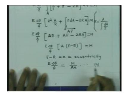
This will give us E delta phi by phi, you will find that these are going to have very simple form. So, it is A R square by R plus this is going to be R. Then, we are going to have minus 2 R. So, that is d A. So, R square by R plus R, this is equal to M E delta phi by phi. I would like you to consider, the point we had already derived that R is equal to A by integration d A by R minus y which is nothing but R. So, that was the relationship.
