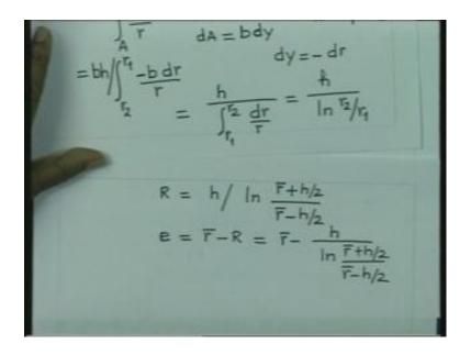
So, you can write in terms of the radius of curvature of this centroidal axis. So, this is nothing but, 1 n. This is r bar plus h by 2 divided by r bar minus h by 2. So, that is the value for the radius of curvature. And the eccentricity is nothing but, r bar minus R. So, we have the eccentricity now given by h divided by 1 n r bar plus h by 2 divided by r bar minus h by 2.
