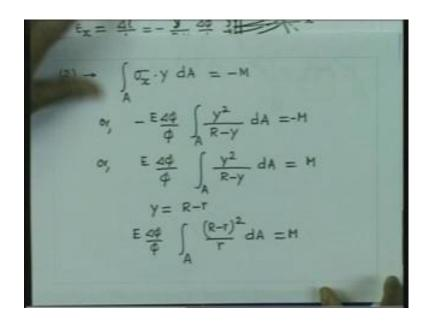
We will consider now the 2nd equation which is nothing but, sigma x multiplied by y d A over the whole cross sectional area is equal to minus M. Or you can write minus E delta phi by phi y square by R minus y d A is equal to minus M or E delta phi by phi y square R minus y d A is equal to M. We can now consider one simplification here or geometries shown ((Refer Time: 34:12)).
