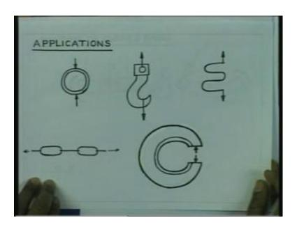
Think of a circular ring. It is subjected to diametrical compression. Think of the hook of a crane, which is curved here. And it is subjected to loading and under the action of the loading, there is going to be bending, developed. Similarly, you comes across pipelines like this, which are subjected to loading. You can also have the press frame c press frame, which is going to look like this. And it is subjected to loading and that is going to cause bending in the portion here.
