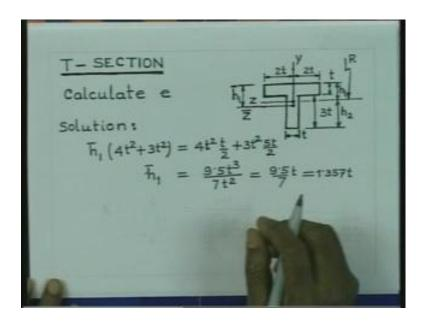
So, let us now consider a T section. So, the section is shown here, that we have 1 t formed by a rectangular portion of dimension 4 t by t and another portion. So, the flange is of dimension 4 t by t and the ((Refer Time: 52:19)) is of dimension 3 t by t. The centroidal axis will pass through the centroid of the cross section. Therefore, in this case it is not obvious, where the centroid is located. So, it has got to be located first.
