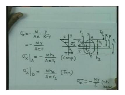
So, if we now substitute the value in that stress relationship, we now find that sigma x is equal to minus M by A e y by R minus y, which is same thing as M y A e into R. The radius of curvature of the fiber. So, what we are considering, that this is the fiber we are concentrating and this fiber has a radius R. So, the stress in this phi bar is given by M into y, where it is located at a distance of y from the neutral axis.
