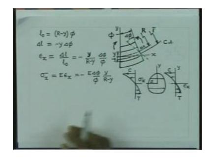
So, that is the portion and this section gets rotated by an angle, this much which we have indicated by delta phi. So, this is the this axis is centroidal axis and this is the neutral axis. So, this one is neutral axis. If we now concentrate on a fiber, which is located here. Please note that we have indicated y axis here and our x axis is located in this direction. So, therefore, this is really the direction of x axis.
