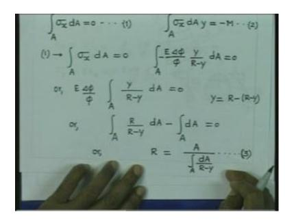
Therefore, the force acting on this fiber is nothing but, sigma x. If you consider that this area is nothing but, d A. Then, sigma x into d A is the force acting on that element. And now if we integrate the total force acting on the cross section. That is going to be sigma x into d A. This particular cross section is only subjected to bending moment in and there is no axial force acting on the cross section. And therefore, we must get the sum of the axial stresses to be equal to 0.
