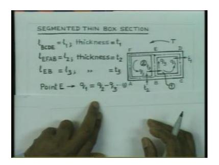
Typically, what we are trying to concentrate upon in sections like this, where we have, one box consisting of these four walls, another box consisting of these four walls. The total torque, that is acting on the section is T. Let us say that, this part or box would indicate by box 1. And this box, which is consisting of the portion, let us say E F, A B E is 2 and here, it is B C D E B is box 1.
