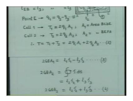
If I consider now this cell number 1. We can write now 2 G theta into area of this cell A 1. That must be equal to integral of this quantity tau into d s. So, we have to take the route B to C, C to D, D to E and again E to B A 1, of course, which is the area enclosed by the contour B C D, E B. Now, let us look into, what this integral is finally, going to lead to, we have the thickness all over the length is constant and the flow is q 1.
