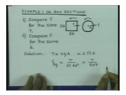
Let us solve, some simple problems, applying this derivation. Let us consider, one example of simple square box sections, where the sides are 2 a, thickness is t. And we have round section, here the radius is a, thickness is t. What you are required to is that; compare the shear stress, maximum shear stress for the same T. In the second case, you are asked to compare the shear stress for the same angle of theta.
