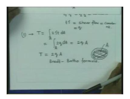
Getting back to relation 1; we have T is equal to 2 times t into tau into t into d A. And this is over the whole cross section. If we represent the shear flow to be equal to q. Let us say, shear flow is q. Then, what we have here, so this is from 1, we have A 2 q, d A and q is constant. So, therefore, this is q and integration of d A is nothing but, A. So, torque capacity is related to shear flow multiplied by this area.
