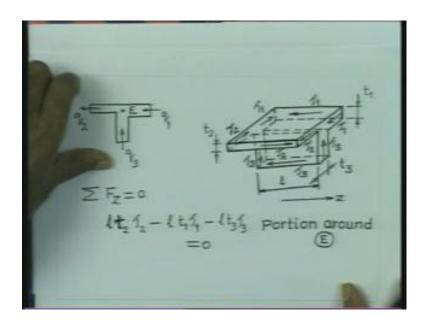
Let us look into, therefore, the point, this is the point that we are talking about. Now, our beam is on the box section shaft is going to be in the length direction. In this direction, I am just trying to take a portion of the section like this. And let us assume, that the flow, since flow is in this direction, it is of magnitude q 1, here it is q 3, here q 2. When, I take this section, the thickness here is t 1 and the shear flow is here in this direction.
