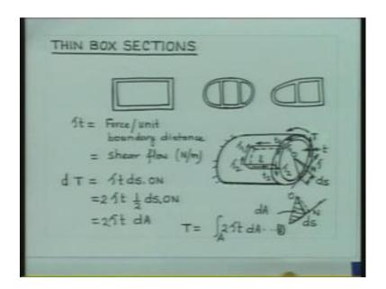
So, it will be oriented in the axial direction. And let us now try to see, the forces, net force on this element in the axial direction. So, if you would like to consider that axial direction is equal to z. This is our z direction. Then, some of the forces on this element; just take it out. And think of it, that forces are acting on this boundary, which are of intensity tau 1 there, tau 2 there.
