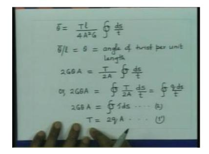
If you consider that the angle of twist of the whole bar is theta bar. So, theta bar, total angle of twist. That we can obtain from, application of Castigliano Theorem, which is nothing but, derivative of u, with respect to the applied stress, which is torque and in this case, it is d U, d T. So, you get now, theta bar is equal to T 1 by 4, A square, G integration of this quantity, d s by t. We like to write this thing, theta by 1 as equal to theta, it is equal to angle of twist per unit length.
