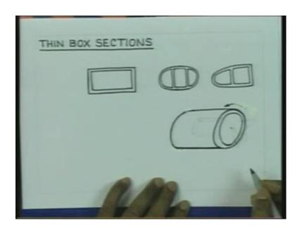
They may look like this, you can have a rectangular box sections like this with thin walls. They need not be uniform, but you could have section like this compartmented or sectioned like this compartmented. If you look into this section, it looks very similar to that of aircraft wing and this could be another section of the aircraft wing. So, these types of sections are utilized in the case of missing tools, bed and also aircraft wings, although we have, other applications too.
