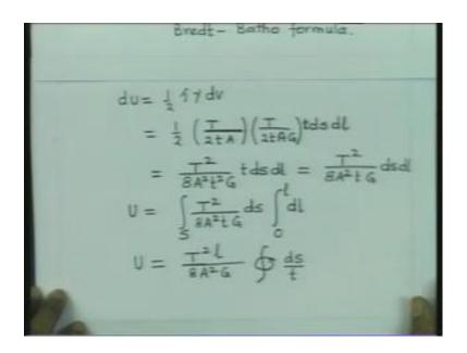
This gives us T square, 8 A square, t square, G, t, d s, d l which is nothing but, T square by 8 A square into t into G, d s, into d l. The total energy is therefore, obtained by integration of T square 8, A square, t, G, d s, over the boundary. And this l is, 0 to l into integration of this. And since we have l can be integrated easily. So, therefore, we have now, T square, t is constant and 8, A square, G and this is integration of the quantity d s by t. So, u is this 1.
