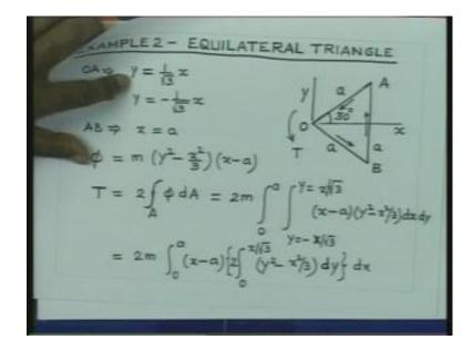
And the dimension is given by a here, the torque is acting in the anticlockwise direction like this. Let us find out, where is the maximum stress. In this case, we expect as usual the stresses to be acting parallel to the boundary. So, we can show the direction of the stresses to be there, like that. The equation of the line O A is nothing but y tan 30 x 1 by root 3 x equation of O B is y equal to minus 1 by root 3 x and A B x is equal to a.
