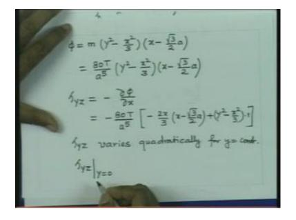
Phi was given as m into y square minus x square by 3 x minus root 3 by 2 into a. Now, if you substitute the value here, 80 T by a 5 x minus root 3 by 2 a. Let us calculate the stress, tau y z which is given by delta phi minus delta phi delta x. So, this will give us minus 80 T by a 5 minus 2 x by 3 x minus root 3 by 2 a plus y square plus x square by 3 into 1. So, that is the variation; and you can see that the stress varies quadratically, quadratically for a particular value of y.
