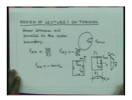
Let us first review our earlier lecture. That is lecture 1 on torsion of non-circular shafts. We have noted few things, that while applying torsion, each section is going to have warping. And that warping is a solution of Laplace equation. And we have noted that the section is subjected to shear stresses, which will have a typical feature. That shear stress cannot be acting normal to the boundary.
