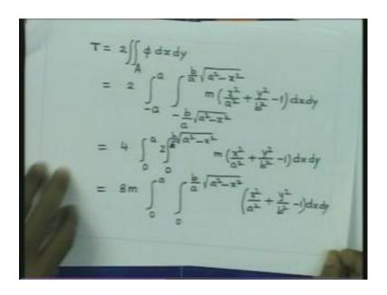
Now, we would like to go in for the utilization of another relationship. That the torque applied is related to the phi surface by this relationship. Integration of the phi function, over the whole area. This is nothing but integration we can now consider that, this integration x is varying from minus a to a. And y is varying from minus b by a, a square minus x square to b by a a square minus x square. And phi is, you can now write the value of phi.
