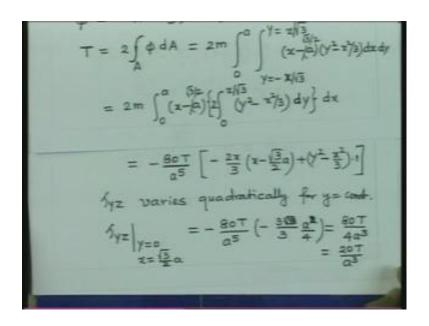
So, tau y z varies quadratically for y constant. Typically if you like to consider tau y z for y equal to 0. And x is equal to root 3 by 2. Let us get back to our ((Refer Time 46:55)) extreme point. So, extreme point is x is equal to root 3 by 2 a. So, if you substitute that, then it comes out to be minus 80 T by a 5. Here, this is going to cancel out and we are going to have minus, it is 3 into root 3 by 3; it is going to be 3 by 3 4 a square.
