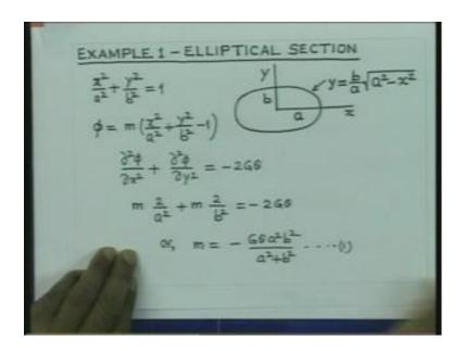
Let us first consider the example of elliptical section. Let us say that the major axis, semi major axis is a, semi minor axis is b. And therefore, this curve is nothing but y equal to b by a root over a square minus x square. The equation of the boundary is given by x square by a square y square by b square is equal to 1. So, the boundary equation is nothing but curve is nothing but x square by a square plus y square by b square minus 1 equal to 0.
