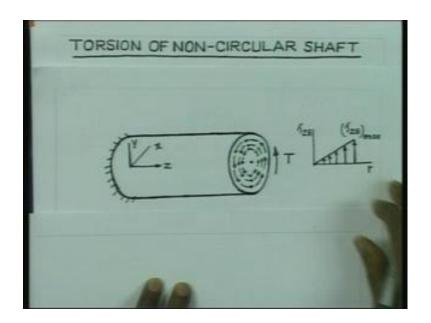
Today, we are going to study torsion of non circular shaft. You have already studied torsion of circular shaft, where you have seen when a circular shaft is subjected to twist. The shaft of uniform cross section will undergo deformation. And a typical cross section of the shaft will give rise to shear stresses, which are going to be distributed like this. The shear stress has a variation with radius, which varies from 0 to maximum value at the outer radius.
