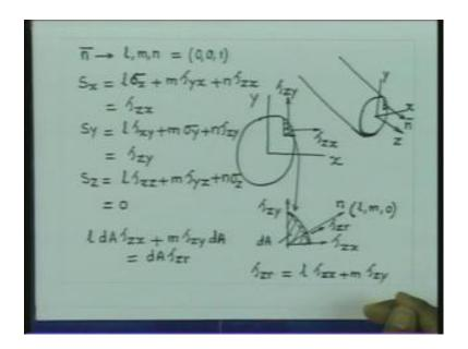
So, this component is going to be like this. I want to note this point very carefully that this tau z r is the stress acting in this direction. And it is really acting perpendicular to the boundary. So, this stress acting perpendicular to the boundary, this is given by this magnitude. And if you now consider, consider an area let us say that, we consider an area like this.
