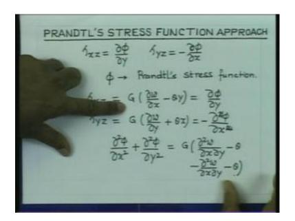
Prandtl introduced one stress function. And he defined the stresses, we had two nonzero component of stresses tau x z. And he defined that, this stress is given by delta phi delta y, where phi is the Prandtl stress function. Similarly, tau y z is given by delta phi delta x. So, phi is Prandtl stress function. Now, we can get some relationship between this
