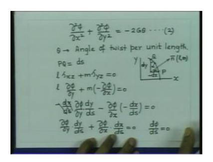
So, delta 2 phi delta x square plus delta 2 phi delta y square is equal to minus 2 G theta. This is an important equation of torsion. So therefore, the Prandtl's stress function is such that, it satisfies the Poisson type equation. Note that, G is a material constant and theta. Theta is nothing but angle of twist per unit length. We will derive certain characteristics satisfied by demonstrated by this Prandtl's stress function. We have already seen that, if I consider the part of the boundary.
