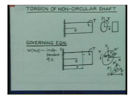
The section as I said it could be elliptical or rectangular. Now, another action of this torsion, the deformation of the shaft will take place. And this deformation will give rise to stresses, at each and every cross section. Now, if you look into a typical cross section of the shaft. Let us consider that, this is the typical cross section and ((Refer Time: 02:33)) apply angle of twist. Angle of ((Refer Time: 02:37)).
