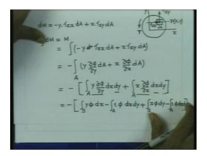
d M is equal to tau z x into d A multiplied by the distance y. So, this is going to be ((Refer Time: 49:47)) y tau z x into d A. That is the moment and this moment is going to be clockwise. So, we are going to write it negative. Then the moment due to tau z y into d A. That is going to be anticlockwise and the moment is x. So, therefore, we will have x tau z y into d A.
