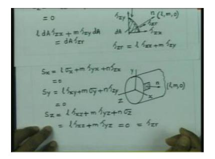
So, this is x axis, this is y axis and this is the one z axis. Now, let us consider an area here. And this area it is outer normal. Let us say, that it is equal to n. And this n could have direction cosine. Let us say I m and since this is in the plane of x and y. This outer normal is in a plane parallel to the plane x and y it is component. The direction cosine
