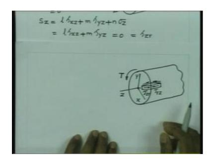
So, I would like you to look into this sketch we are considering this element. It is oriented in the r z plane. So, this is your r direction. And this is your z direction. The z r stress is going to act on this plane. Similarly, the pair of this is going to be directed towards the center. And the complementary shear stress, if you are going to come up on this stress it will be oriented like this. And on the other phase it is going to be oriented like this.
