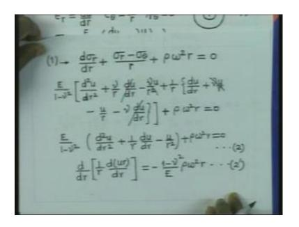
Now, we have to solve for this equation. We make use of the values of sigma r and sigma theta. So, therefore after substitution we will have the following. So, that is d sigma d r. And then we can also go on substituting the value of sigma r and sigma theta here. So, therefore we will have E by 1 minus nu square can be taken out. And we will be left with d u d r plus nu u by r minus u by r minus nu d u d r plus rho omega square r equal to 0.
