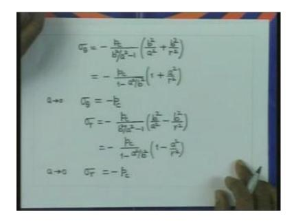
So, if we just consider now the formula that we have derived for sigma theta. Sigma theta for an externally pressurized cylinder was like this. If it is having b and a as the radii, then we have the formula like this. This is the variation and it is all compressive. Now, the shaft represents a case with a equal to 0. So, if we put a equal to 0, it will leads leads to infinity. And it is not possible to get the solution for the solid cylinder.
