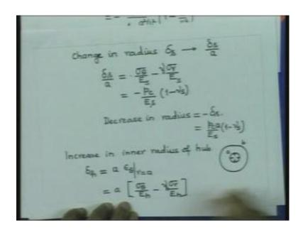
Let us say, change in radius of shaft is delta s. And therefore, this strain is going to be delta s by a. That is the strain. And therefore, this strain is equal to it is given by Hooke's law sigma theta by E minus nu times sigma bar by E. And if you would like to add the subscript for the shaft is. So, therefore we will have this value. Now, since both are minus p c. So, therefore what we have here is p c by E s into 1 minus nu s. That is the change in radius.
