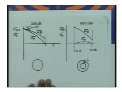
You have both sigma theta sigma r equal to 3 plus nu by 8 rho omega square into b square. So, the magnitude of the value here, at this point we can write the value. It is 3 plus nu by 8 into rho omega square into b square. That is the value of the stress. And the radial stress is zero at the outer radius. And the sigma theta stress is going to be higher than that. So, therefore this is the value here.
