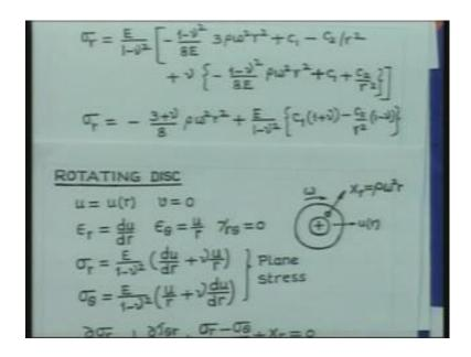
And this disc, when this disc is rotating what do you expect to be your radial stress at the inner surface, so also at the outer surface? The material which is just lying on the right of this inner surface is trying to move up, radially outward. So, therefore it will be pressing the material lying to the right of it. But for the outer surface, there is no material lying on the left of it. So, therefore there is no radial force acting the surface.
