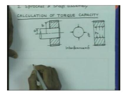
Now, under the action of the shrink fitting there will be some contact pressure acting on the shaft. Let us say that is p c. And the same p c is going to act on the surface of the inner surface of the gear hub. So, we can imagine that the gear hub is going to be subjected to the same pressure. So, this same pressure is going to act here. Depending on the initial interference, it is possible to calculate the pressure p c that you have noted already.
