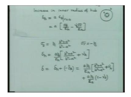
We can now see that, sigma theta is nothing, but p c is the contact pressure. Therefore, this sigma theta is equal to p c into b square plus a square by b square minus a square. And sigma r is equal to minus p c. Therefore, we will have delta h is equal to a into p c by E h b square plus a square by b square minus a square. And this is going to be minus gamma h. So, we have both got both increase in the radius of the hub and also the decrease in the radius of the shaft.
