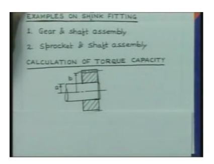
Shrink fitting is can be made use of in assembling a gear on a shaft. And when you are trying to do this, it is sometimes necessary to calculate the torque capacity. Along similar lines, some time sprockets are mounted on shaft using the shrink fitting. One advantage you get in this process is that, you can do away with the key way, the key of ways. So, you do not need to have the keying for the sprocket on the shaft or the gear on the shaft.
