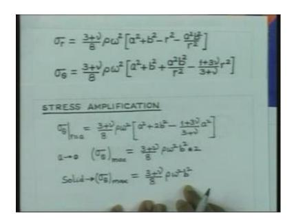
So, if you now consider this hoop stress as we have considering the stress at r equal to a. So, at r equal to a sigma theta at r equal to a is going to be given by 3 plus nu by 8 rho omega square. So, r equal to a means, we will have a square plus 2 times b square minus 1 plus 3 nu by 3 plus nu a square. So, that is the stress at the inner radius of the disc. Now, when you are trying to say that a is very very small, a is tending to 0.
