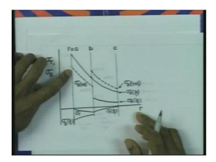
So, once this contact pressure is calculated, it is very easy to calculate the distribution of stresses in the duplex cylinder in the assembly. So, we would like to show those stresses. The radii, let us say that a is the internal radius b is the common radius c is the external radius as we have considered the symbol earlier. The internal cylinder is going to be subjected to external pressure loading.
