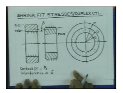
So, if we have such construction they are sometime called as duplex cylinder. And the assembly is done by shrink fitting. So, if you consider a duplex cylinder to be made up of two cylinders. Like this one of radii a and b, another of radii b and c. In this case, the inner cylinder has been fitted into the external one, to get this composite cylinder or duplex cylinder. Now in order to do that, we go for shrink fitting.
