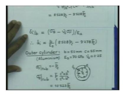
So, the strain that is going to develop in the circumferential direction is nothing but delta i by b. And that should be given by the relationship sigma theta minus nu s into sigma r divided by E s. Again, if you substitute if you just actually write now. Delta i is equal to
