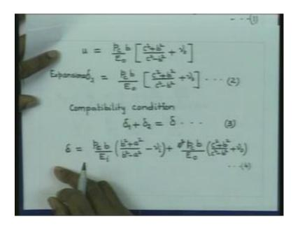
Compatibility condition delta 1 plus delta 2 is equal to delta. We have already seen that delta 1 and delta 2. They are functions of contact pressure and the dimensions of the cylinder plus the material constants. And we know, all the quantities accepting this contact pressure. So, therefore by substituting in this relationship we get an equation involving the interference and the contact pressures. So, therefore this gives us.
