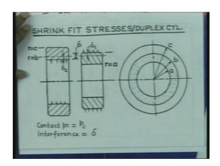
So, this diagram it shows that under the action of the contact pressure, the outer wall of the inner cylinder is going to get contracted. And it is going to move by a distance delta 1. This is delta 1. Similarly, under the action of the same contact pressure, the inner wall of the outer cylinder is going to get expanded by this amount delta 2. So, therefore the initial interference if the two cylinders attain a common radius likes this.
