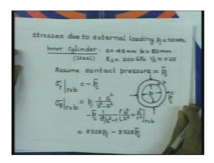
What you can consider here? Just think of the existence of the inner cylinder if the internal pressure p i is acting. Then, the cylinder will expand both a and b will increase in value. And since, after this radius the aluminium cylinder is existing the free expansion of the dimension b cannot take place. So, there will be some restraint on the expansion.
