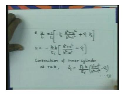
Therefore, u by b is equal to sigma theta already we have the value as r equal to b. So, we can substitute the value. So, we will have 1 by E i common here. And then in that substitution of sigma theta will give us minus p c b square plus a square by b square minus a square minus nu i into sigma r, sigma r is minus p c. So therefore, it will be nu i multiplied by p c. So, that gives us the value of the strain at r equal to b.
