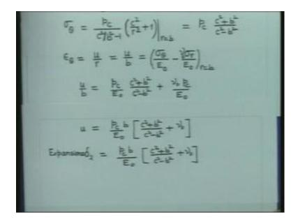
Finally, we get the radial displacement u at r equal to b given by p c by E 0 into b multiplied by c square plus b square divided by c square minus b square, nu 0 plus nu 0. So, that is the value of the displacement. Here in, you find that this is positive quantity greater than 1, this is positive quantity and these are all positive. So, therefore u is positive.
