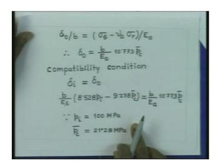
Obviously, this strain which is in the circumferential direction, it is given by delta 0 by b equal to sigma theta minus nu a into sigma r by E. And if we again substitute these values, here we get this much. So, the compatibility condition here is that. The expansion of the outer radius of the inner cylinder delta i must be equal to the expansion of the inner radius of the outer cylinder.
