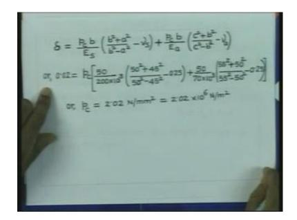
So, if we substitute now the value we will keep it all in Newton millimeter units. So, therefore it is 0.02 is equal to p c into b is 50 divided by modulus 200 into 10 to the power 3. It is in Newton per millimeter square. The dimension b here is 50, a here is 45. The Poisson's ratio is 0.25. Similarly, in this case b is 50. Modulus is 70 into 10 to the power 3.
