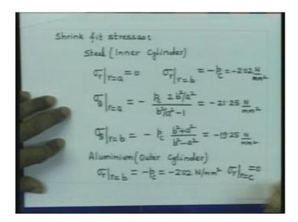
So, we will now calculate shrink fit stresses. Let us first consider the steel cylinder which is nothing but the inner cylinder. It is subjected to radial pressure from outside. So, therefore sigma r at r equal to a is 0 sigma r at r equal to b equal to minus p c, which is nothing but minus 2.02 Newton per millimeter square.
