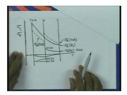
But then in this case, since the material of the inner cylinder is of steel and that of the outer cylinder is of aluminium, we have to have a different approach. So, let us now see how we can calculate these stresses.
