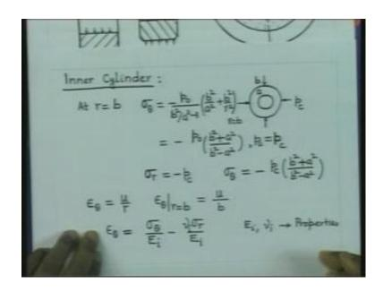
So, let us consider inner cylinder. So, the inner cylinder is subjected to pressure at its outer boundary. So, we have the inner cylinder with radii a and b. Now, in the assembly the inner cylinder is subjected to contact pressure p c. Therefore, we can find out the stress in the inner cylinder. Particularly, at r equal to b. We have this stresses sigma theta and that is given by the formula. Just now or the formula that, we have derived in the earlier lecture.
