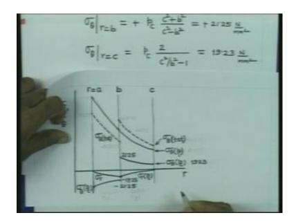
Then we have sigma theta at r equal to b. This is given by p c c square plus b square divided by c square minus b square. And this is of magnitude mi this is of course, positive. So, this is 21.25 Newton per millimeter square. And sigma theta at r equal to c is going to given by 2 times p c divided by c square by b square minus 1. And once you simplify this, this comes out to be 19.23 Newton per millimeter square.
