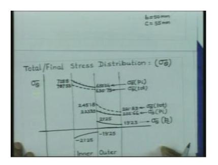
We have a picture like this. The stresses due to the internal pressure, is going to vary like this in the inner cylinder. And the stresses due to the internal pressure, is going to vary like this in the outer cylinder. So, this is the variation of the stresses in the inner and outer cylinder. So, the values are 728.8 and this is 650.04. And this is 223.93 and this is 202.66. So, these are the stresses due to sigma theta due to p internal.
