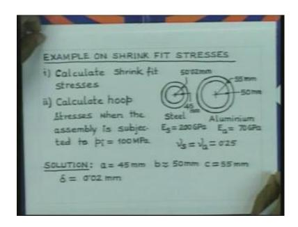
Let us consider this example. We have a steel cylinder of radii 45 millimeter and 50.02 millimeter. And we have aluminum cylinder whose radii are 50 millimeter and 55 millimeter. Now, these two cylinders are assembled together to make a duplex construction. The steel properties are given by modulus 200 GPa and its Poisson's ratio is 0.25. So, we would like to represent the modulus by E s and the Poisson's ratio by nu s.
