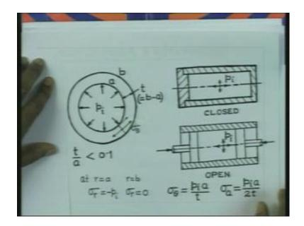
So, if we consider a situation like this, internal pressure is pi internal radius is a, external radius is b. When this wall thickness divided by the internal radius is less than about 0.1 it is called thin cylinder. And you know that when you have such thin cylinder, they are subjected to circumferential stress or hoop stress, given by pi into a by t. And the axial stress is given by pi a by 2 t.
