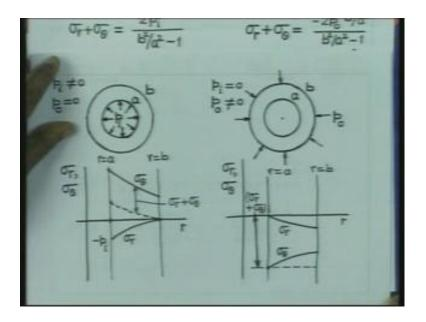
Let us plot the radius in this direction. So, we are considering this is the situation pi is not 0, p 0 is 0 and we have the radial direction. So, radius is plotted in this direction and we would like to plot the stresses sigma r and sigma theta in this direction. Then we have the internal radius is here. So, therefore, this is the internal radius. So, this is r equal to a let us consider that, this is the external radius r equal to b. ((Refer Time: 47:21))
