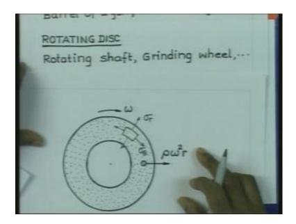
So, you think of a situation like this, that you have a grinding wheel which is mounted on a shaft, it is rotating at some angular speed omega. Then each point of the rotating disc is subjected to centrifugal force. Whose intensity is going to be given by rho omega square into r; where rho is the density of the material, omega is the angular velocity and r is the distance of the point from the centre of the disc.
