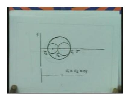
So, let us say that we have the Mohr circle diagram like this in three dimensions. And we have indicated that this is the sigma axis, this is the tau axis and now the stresses are sigma 1 sigma 2 and sigma 3. So, these are the three principle stresses. If the three principle stresses are equal then Mohr circle is going to be one point, so the case, wherein sigma 1 equal to sigma 2 equal to sigma 3 that becomes a point.
