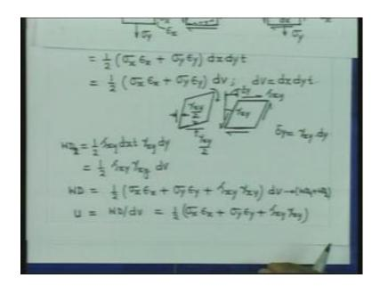
So, if we draw this same component I think, I would like to show that one separately. So, we have this. So, this angle this angle, this is gamma xy by 2, these angle is also gamma xy by 2. Now, by turning this in this direction what we have achieved is that this angle is equal to gamma xy. So, therefore, if we now consider the stresses acting here, this is how the stresses are acting on this element.
