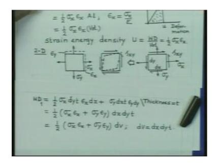
Now, if we consider two dimensions, we will have three components of stresses, sigma x, sigma y then we are going to have shear stresses, which we indicate by tau xy. The two normal stresses, they are going to produce normal strains and this shear stress is going to produce shear strains. Note that this shear stress is not going to produce any normal strain. So, therefore, the work done by the normal stresses and the shear stresses can be calculated separately.
