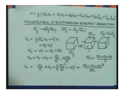
So, in three dimensions you will find that this strain energy density U is going to involve all the 6 components of stresses and strains and it will be like this sigma half into sigma x into epsilon x sigma y into epsilon y plus sigma z epsilon z plus tau yz gamma yz tau zx gamma zx plus tau xy into gamma xy. So, that is the form of the energy in three dimensions. Now, we would like to consider that this total strain energy density can be
