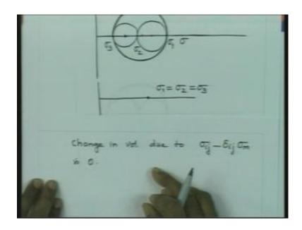
So, therefore, the change in volume, in volume due to deviatory part that is sigma ij minus delta ij sigma m is 0. So, I would like you to derive this relationship. It is very simple that change in volume is due to the normal stresses and in this case three normal stresses are going to be sigma x minus sigma m sigma y minus sigma m sigma z minus sigma m.
