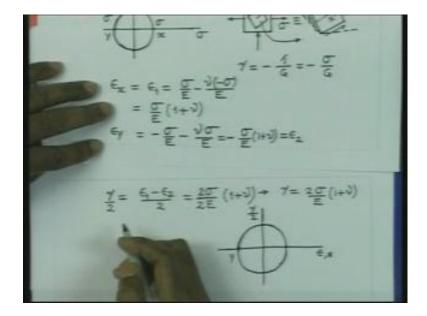
So, epsilon x and in this case, this is the maximum principle stress, this is the minimum principle stress. So, therefore this is epsilon 1 which is nothing but sigma by E or sigma x stress is sigma, sigma by E minus nu times sigma y by E and that minus sigma y is nothing but, minus sigma. Therefore, this divided by E and hence this is equal to sigma by E multiplied by 1 plus nu.
