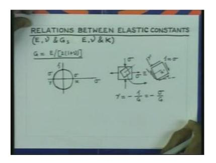
So, first we will try to derive the relationship between G on one hand, E and nu on the other. So, this relationship is of this form, so we would like to derive this relationship. To do this, let us consider a state of stress at a point in a material which is isotropic. This material point is subjected to stresses. Let us say sigma in the x direction and sigma in the y direction, but this is compressive, there is no shear stress. So, therefore, these are principle directions.
