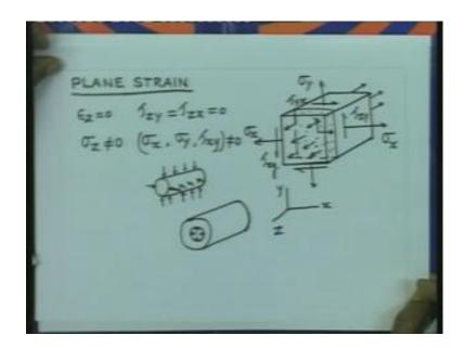
We will consider the other condition which is plane strain condition. If you consider the thick plate and it is if you now have the load of this component by loading like this. We will have sigma x sigma y. And we can also have the shear stresses. And the bottom phase, we can also have the stresses, of course this side we have sigma x and this is tau x y. So, these are the stresses on the phases.
