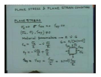
Therefore, the stresses which are going to be 0 are nothing but sigma z equal to 0 and sigma z x equal to 0 and z y equal to 0. These three components are 0. The non-zero components are going to be sigma x sigma y and tau x y. So, these are the three non-zero components. And this particular state of stress is known as plane stress. So, this state of stress is known as plane state of stress. Let us find out the relationship between the stress and strain in this case.
