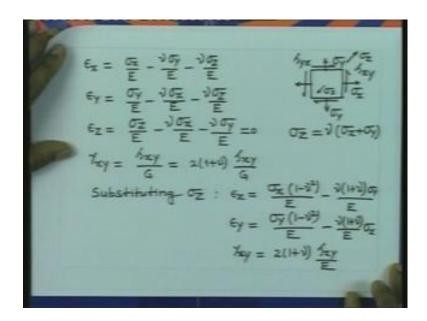
So, a typical element here is going to be subjected to stress like sigma x sigma y. And then, we have shear stress tau x y and tau y x. And also, we have the stress acting in the z direction which is sigma z. The normal stresses will produce normal strain and the shear stresses will produce the shear strain. That is going to valid, if we assume the material to be isotropic.
