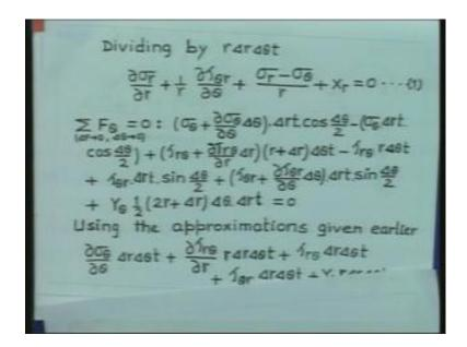
Now, we will consider the equilibrium equations in the Tangential direction. So again, we write some of the forces in the theta direction are 0. And assuming that delta r is very small tending to 0. So also, delta theta is very small. So, delta r is tending to 0. So therefore, if you consider the argument similar to, what we have done earlier.
