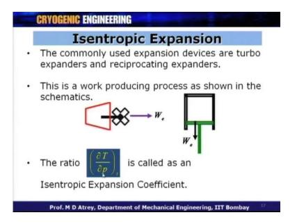
The commonly used expansion devices are turbo expanders which is a turbine for isentropic expansion or reciprocating expanders where cylinder and piston arrangement could be used to cause isentropic expansion. This is a work producing device; now, this is a difference between a J - T expansion and an isentropic expansion. Here in this case, when expansion occurs, there is some kind of work gets produced and we will get some work from this expansion.
