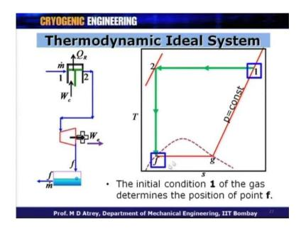
So, if I were to represent this system on a T - S diagram, this would look like this. These are two pressure lines and this is starting point at point 1 over here. So, 1 to 2 process is a isothermal compression process, temperature remains constant. And after pressurization at point 2, here the gas is expanded isentropically, therefore entropy remains constant. And this gas after expansion hits this end which is a such as a liquid curve at this point.
