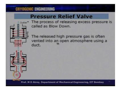
The process of realizing excess pressure is called as blow down. So, blow down will will happen as soon as the set pressure gets exceeded, this seat will go up, and the gas will get blown outside. The released high pressure gas is often vented into an open atmosphere using the duct.
