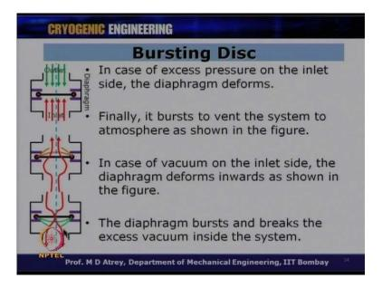
Now, how does it work? In case of excess pressure on the inlet side, the diaphragm deforms. So, we have got a inlet pressure from this side now, and diaphragms takes this
