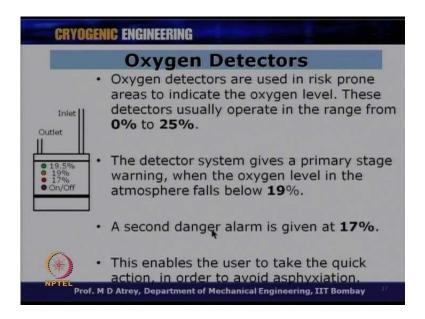
But we should have oxygen detectors. In addition to all these things, what we just talked about, we should have oxygen detectors, which basically detect the percentage of oxygen in the atmosphere around you, which is very important. So, oxygen detectors are used in risk prone areas to indicate the oxygen level. These detectors usually operate in the range of 0 to 25 percent, we know that 19.5 percent is a cut off and therefore, oxygen should be you know indicated from 0 to 25 percent.
