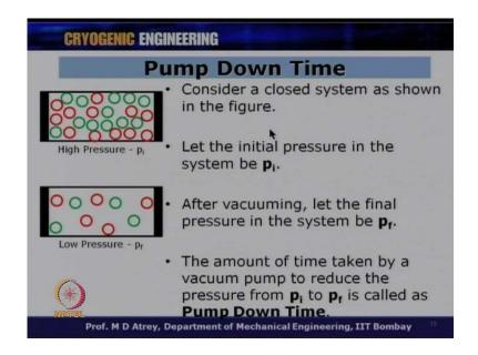
So, consider a closed system as shown in the figure, this is my high pressure to begin with, let the initial pressure in the system be P i, before I started vacuuming my pressure is going to be initial pressure which is P i, and after vacuuming I reach final pressure which is p f. So, I can see that less number of molecules over here, and this is my completely low pressure which I have got after vacuuming from P i to p f.
