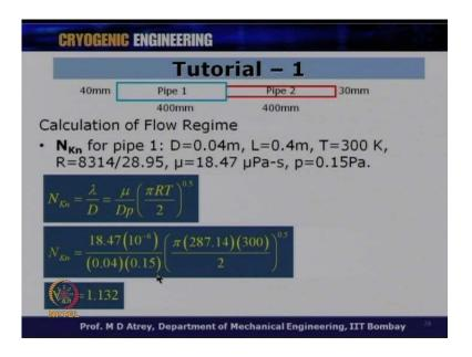
So, calculate the overall conductance C o, calculation of flow regime first in order to ensure in which flow regime I am, because depending on the flow regime I have to use the expressions for conductances.
