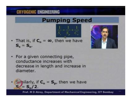
So, when C o is infinite what we get is this, if C o is infinite then we have S s is equal to S p. Can we have C o as infinite, is it possible? We will see that later.
