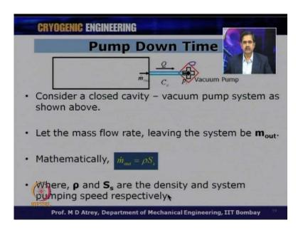
So, let us see this system, so considering the close cavity as shown over here with the vacuum pump system. So, you got a entire thing will be vacuum pump system a close cavity connected to a vacuum pump through a given conductance all right.
