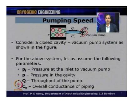
Now, let us come to know what this pumping speed is. So, what we can see here is a cavity or a cylinder which is shown to be vacuumed, and there is a vacuum pump kept on the right, the vacuum pump is a is a known device to me and therefore, vacuum pump will have known characteristics; however, this vacuum pump is directly not mounted on the system to be vacuumed, but it is connected to some piping arrangement and therefore, the conductance of this pipe also become very important.
