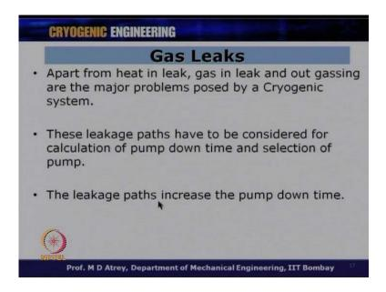
Now, this parameter will also depend on what are the leakages paths? The gas is going to get leaked over a period of time, and the gas is going to get leak leakage paths could be definitely there, as long as the fabrications happen you got always joints, you got some seal matters, you got a material which out gases and therefore, gas leaks is always going to be there.
