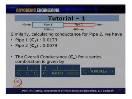
Similarly, calculate conductance for pipe 2 now, we got again pipe 1 as C 1 0.0173 and pipe C 2 we get 0.0079. The conductance for point the pipe C 2 is quite less as compared to what because the diameters are different.
