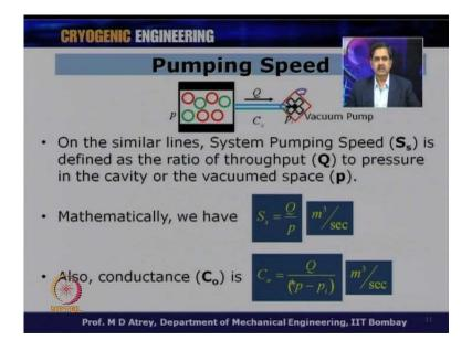
On the similar line this is a system pumping speed. So, we got a vacuum pumping speed which is the pumping speed normally refer to as, and then we had a system pumping speed which is specified for the system here, this is my system to be vacuumed, this is my vacuum pump I have been utilized, and this is the way I have connected this vacuum pump to the system.
