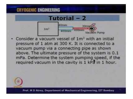
Now, tutorial is, if this arrangement what we have just seen is connected to vacuum a system of 1 meter cube volume, and I got a vacuum pump at the other end over here. So, now I can see that I got a entire system, which are known conductance which we are just calculated with the vacuum pump on one side, and system to be vacuumed on the other side.
