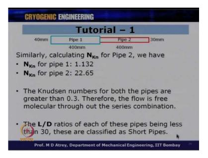
Similarly, I can do it for pipe 2 also, similarly calculating for Knudsen number for pipe 2 what we have is, Knudsen number of pipe 1 is 1.132, and Knudsen number for pipe 2 is 22.65 which is very high, we are not shown the calculations again and therefore, you can see that Knudsen number has been directly calculated for the pipe 2.
