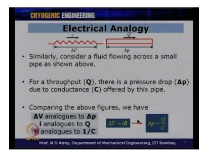
Now, can we compare this electrical circuits of having voltage difference across a given resistance of length l through which a current I flows. So, now, let me compare this with a pipe and this I say that a pipe flow occurs Q which is comparable with I and this Q occurs only when the delta p occurs across the length of the pipe and the length of the pipe is l and delta p is the pressure drop across the length of the pipe l.
