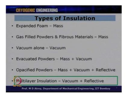
So, these where the insulation which we had talked about of which we had studied all this first 5 cases; what we are going to learn now is about multilayer insulation; which basically have vacuum, which works in vacuum and also which has got a reflective medium also. So, right. So, here we will talk about multilayer insulation now in this particular lecture. So, let us see what is this multilayer insulation is all about.
