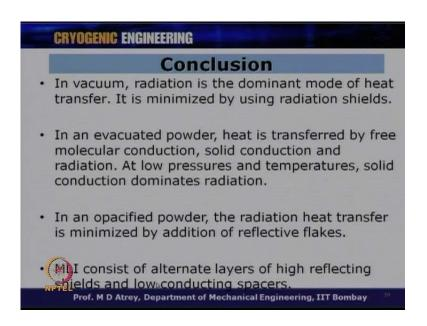
In vacuum, we have seen that the radiation is a dominant mode of heat transfer and it is minimized, it can be minimize using radiation shield. But we know that having radiation shields, it will not be a practical solution for various cryo containers. In an evacuated powder, heat is transferred by a free molecular conduction, solid conduction and radiation. At low pressures and temperatures solid conduction will dominate the radiation sorry it will dominate the mode of radiation heat transfer.
