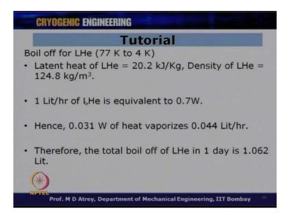
If I want to calculate now the boil off of liquid helium, because of this, I will take into consideration the latent heat of liquid helium which is only 20.2 kilo joule per kg, density of liquid helium is 124.8 kg per meter cube. And we know from the earlier calculation
