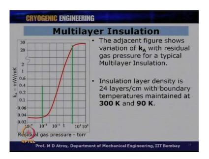
So, multilayer insulation now, the adjacent figure shows the variation of apparent thermal conductivity for multilayer insulation with residual gas pressure. So, basically this will tell you what is the effect of vacuum on the apparent thermal conductivity for a typical multilayer insulation. So, you can see that insulation layer density is 24 layers per centimeter in this case and a temperatures are 300 K and 90 K for which the values are given over here.
