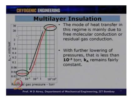
If you go further down from now; the mode of heat transfer in this region will be made mainly due to free molecular conduction or residual gas conduction alright. Radiation will be taken care of, because of multilayer insulation. But will have a gas conduction now which is very, very important to be minimize by lowering this vacuum.
