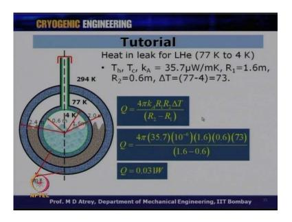
So, heat in leak calculations again would be done; delta T is going to be 77 minus 4 is 73 kelvin. R 1 and R 2 are going to be different, R 1 is 1.6 meter and R 2 is 0.6 meter. If I put this values in the same formula now, I will get Q is equal to 0.031 watts. That means only 31 milliwatt is going to be by heat in leak from 77 kelvin to 4 kelvin.
