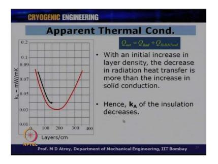
So, layers per centimeters given here which is nothing but N by delta x. Against which we found a apparent thermal conductivity and you can see that this kind of variation is shown. And we can see that at a particular number of layers per centimeter, we can have minimum k A value in milli watts per meter Kelvin. Why does it happen?
