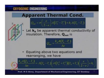
Let us now find out what is apparent thermal conductivity for multilayer insulation. Let k A be the apparent thermal conductivity of the multilayer insulation and therefore, Q net in this case is equal to k A into A into T h minus T c upon delta x. Equating this two parts I will say k A into A into T h minus T c upon delta x is equal to what Q net we got over here alright.
